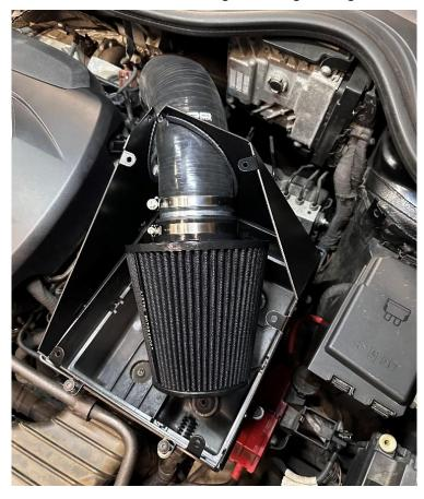
8. Using three supplied plastic push fittings, the two halves can now be secured together.
