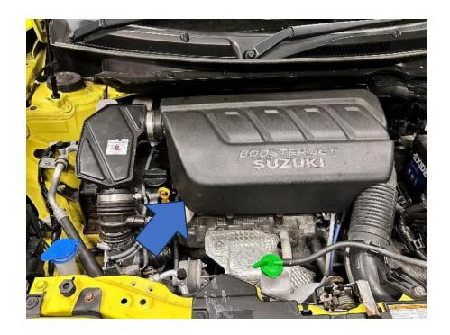
2. At the back of the engine bay, locate the air feed and disconnect it from the back of the air box and the hard plastic pipe at the front. There are two small hoses that are attached to the back of the hose that you will need to disconnect as you take the hose out of the engine bay (blue arrows show position).
