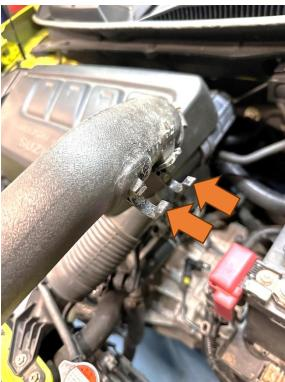
6. Undo the jubilee clip attaching the silicone hose to the intercooler. You may need to remove either the under tray or bumper to gain access to this. Please refer to the AIRTEC Motorsport intercooler fitting instructions to remind yourself of these steps, if required.
