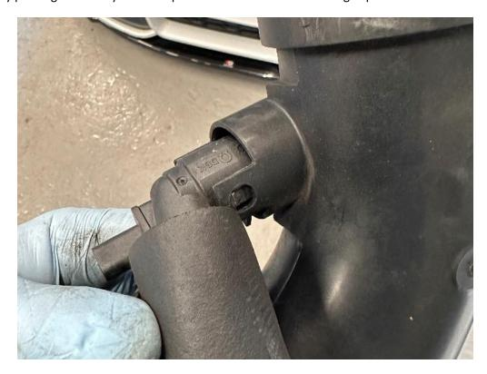
13. The retaining clip can also be removed from the original pipe by pulling it up. Install it onto the new AIRTEC Motorsport pipe but don't let it fully click into place otherwise you will not be able to install the pipe.
