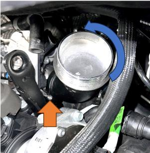
6. Reinstall the hose and bracket removed in Step 3 using the supplied M6x12mm bolt with washer. Then reconnect the plug for the actuator and the wiring loom clip removed in Step 2.
