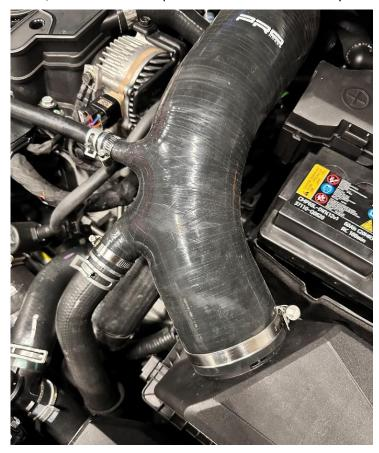
8. **Please note:** if your car is fitted with an AIRTEC Motorsport catch can, the increase in hose size hose at the back of the engine will mean you need to reroute the rear catch can hose over the top of the silicone induction pipe and use a 90-degree push fitting to attach it to the catch can; please get in contact if you require one.
