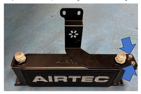
11. Locate the oil cooler onto the car by placing the top bracket onto the two threaded holes as shown. You can then install it using the supplied M6x25mm Socket Head bolts with large washers, but do not fully tighten yet.
