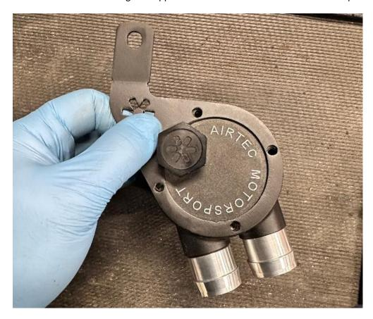
4. Install the catch can assembly onto the car using the supplied M6 bolt, Nyloc nut with washers to secure.
