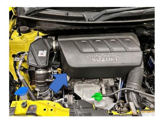
2. Locate the original oil breather hose and using the hose clamp pliers move the hose clamps so that the hose can be removed from the car.
