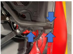
2. Now peel back the rubber trim and undo the four 15mm bolts on each side.
