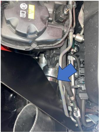
20. Now fit the supplied CNC joiner into the remaining air filter and tighten the jubilee clip. You can then push the connector into the silicone hose together with the last supplied jubilee clip and fully tighten.
