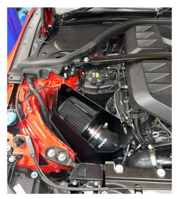
22. Finally, add the air box lid using the last four push fits and refit the sturt brace in reverse of removal.
