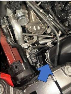
7. To allow extra clerance to remove the pipe from the engine bay, lift the bottom right-hand side corner of the engine cover off of its rubber mount and also undo the wiring plug (blue arrow).
