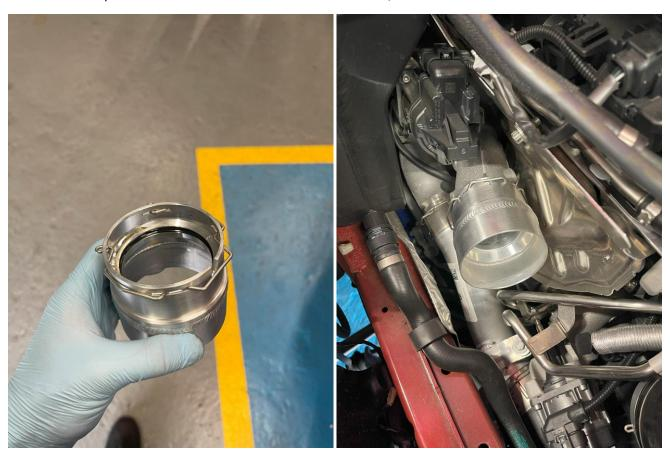
18. For the second air box, only fit the **rear** part of the induction shield using the supplied bolts. You can then refit it back into the car, as shown.
