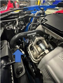
14. When reinstalling the lower front plastic undertray, use the supplied M6 bolt and washer instead of the original push fit at the point shown, as this will secure the turbo radiator from below.
