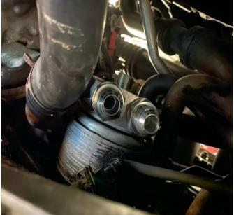
10. You can now connect the oil lines to the sandwich plate. Make sure they are fully tightened before refitting the oil filter.
