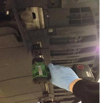
4. Unclip the bumper each side by firmly but carefully pulling it away from the wings.
