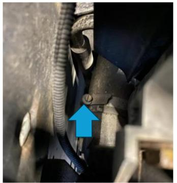
6. Now undo the two 13mm bolts at the top of the intercooler.
