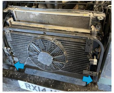
8. With the intercooler removed you will need to trim the plastic blocks from each side of the radiator using a Dremmel tool, hack saw or similar.
