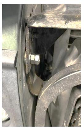
4. At this stage, you will need to find a support for the bonnet. You can then remove the four 8mm bolts (two each side) holding the brackets in place. On the left-hand side, the top bolt undoes the bracket that supports the air conditioning pipework. This cannot be removed, so just slide the bracket up the pipe and out of the way.
