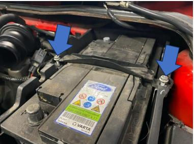
8. Now remove the battery and then remove the plastic clip and 8mm screw securing the wiring harness plug to the side of the battery tray. Remove the three 10mm bolts inside of the battery tray to release it. You will see four 15mm nuts underneath where the tray was located; remove these so you can allow the bracket to turn and allow enough space for you to remove your pipework.
