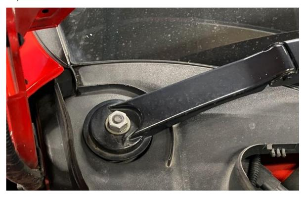
6. You can now remove the upper scuttle panel, which will give access to the lower panel. Remove the 10mm bolt each side to allow this panel to be released.
