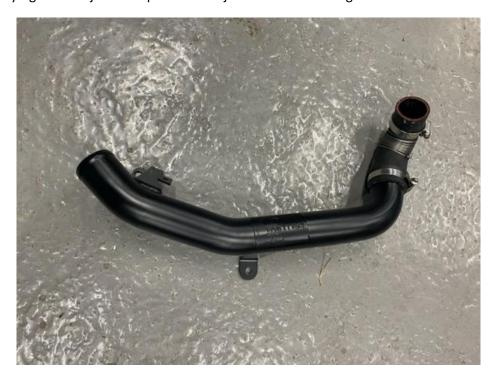
10. Finally, install the pipework in reverse of removal and once in place fully tighten the rear jubilee clips. Then refit the battery, battery tray, scuttle panels and air box.
