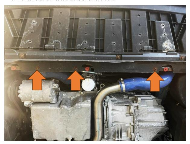
4. Remove the two screws attached to the arch liners.
