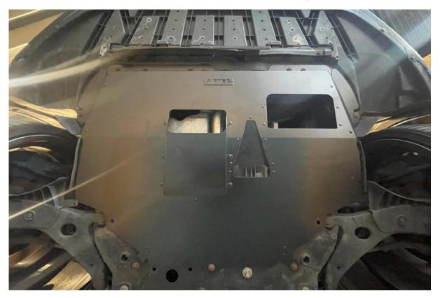
8. Use the supplied bolts and nuts with washers to secure each side of the undertray through the hole left by the plastic inserts removed in Step 5.
