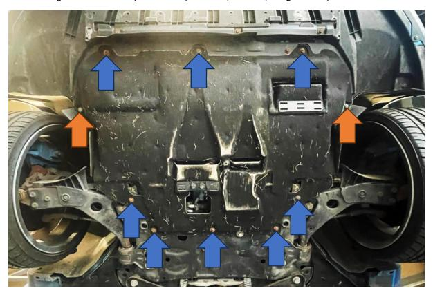
2. To remove the undertray, unhook the centre section (blue arrow).
