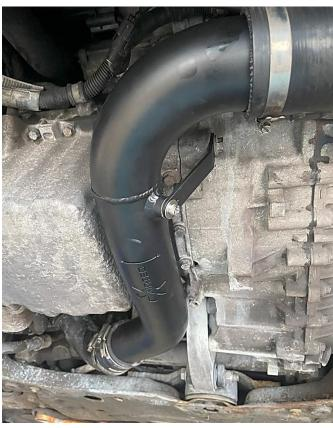
2. Bracket Two attaches to the rear of the gearbox using the same process; do not remove the bolt, simply loosen and slide the 90-degree, U-shaped bracket under the bolt. Then use the second supplied M6 bolt and washer to secure to the pipe. Once in position, fully tighten both the bolts for both brackets.
