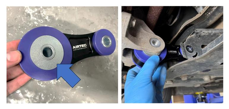
4. Finally, reuse the original bolts and fully tighten. The undertray can then be reinstalled in reverse of removal.
