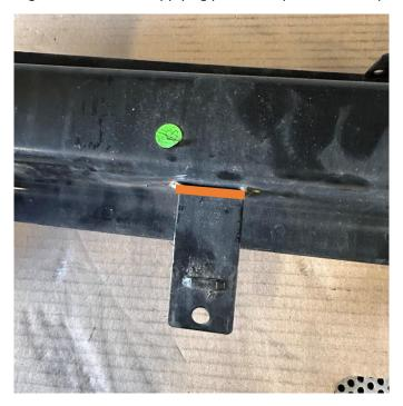
19. Reinstall the crash bar onto the car and install the supplied temperature sensor bracket to the lower right-hand side Torx bolt. Align all of the bolts with the witness marks from where they were previously mounted. This will help to keep the alignment the same.
