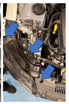
6. Using a pair of axle stands, support the bottom of the plastic radiator cradle.
