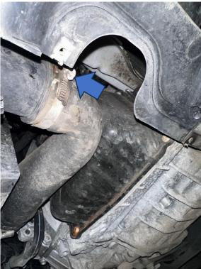
12. Undo the two T27 each side of the radiator cradle. **Please note:** You will need to find a way to support the bonnet before completing this step.
