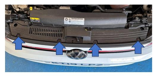
4. With the help of a second person, pull the corner of the bumper out each side, as the bumper comes forward you will need to disconnect a wiring plug on the left-hand side followed by two wiring plugs on the right-hand side and single plug in the middle behind the badge.
