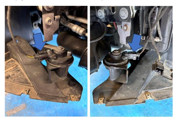
8. Remove the upper front plastic bumper support by undoing the two T25 bolts on top followed by the T27 bolts located each side of the radiator. Then unclip the wiring harness as you remove the surround.
