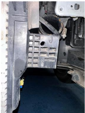
17. With the holes drilled you can now install the intercooler and clip the radiator cradle back into the radiator assembly. Install the brackets using the supplied M6 Hex head bolts with washers and Nyloc nuts and reattach the boost hoses. Position the brackets so that the radiator and the intercooler are not touching and then tighten.
