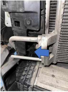
16. The new intercooler can then be test fitted onto the car. Start by installing the brackets loosely with the supplied M6 bolts and washers and push the radiator cradle back onto the radiator assembly and then line them up on the radiator cradle and mark the point where you need to drill. Undo the radiator cradle again and remove the intercooler to allow access to drill the previously marked holes, we recommend using a 7.5mm drill bit.
