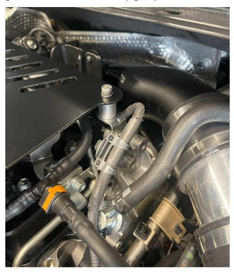
6. Place the remaining boss in the front hole location, as shown and attach it using the remaining bolt and washer. Do not fully tighten yet.
