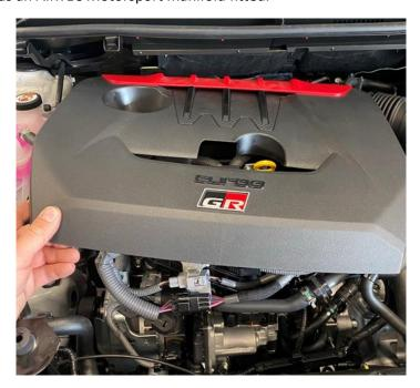
2. Locate the mounting posts as shown. (Cars with an original inlet manifold will have a fourth post on the inlet manifold that is not shown here).
