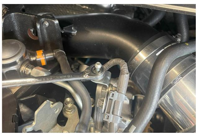
4. Place the longest boss (52mm) in the left-hand side location, as shown, and rest the engine cover over the top. Now screw in the compatible M6x65mm Socket Bolt with a washer but do not fully tighten yet.
