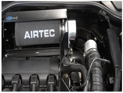
5. Install the air guide blank on the left-hand-side of the air box using the supplied M6 Button Head bolts with washers. On the right-hand side, secure the filter adapter onto the side of the air box using the supplied M6 Button Head bolts with washers. You can now also install the silicone pipework from the alloy pipe connector to the filter adapter.
