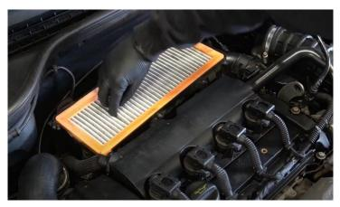
3 Install the AIRTEC Motorsport air box by sliding the three tabs on the back of the air box into the three inserts in the original airbox, then secure in place using the two provided self-tapping screws and washers.
