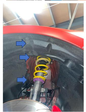
3. Remove the wheel arch and place it in a workable area.
