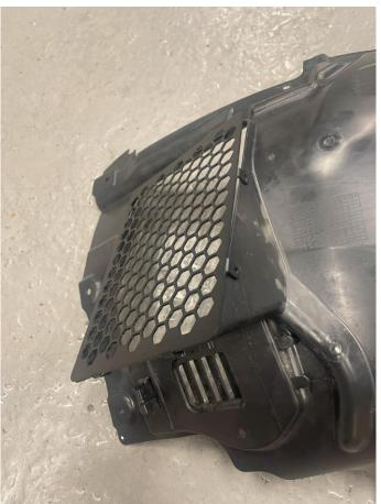
6. Remove the grille and drill 5mm holes in the marked locations.
