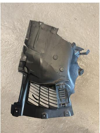
4. Remove the original grille from the arch liner. This can be done with a variety of tools; a Dremel tool, sharp knife, small hacksaw or side cutters will all work.
