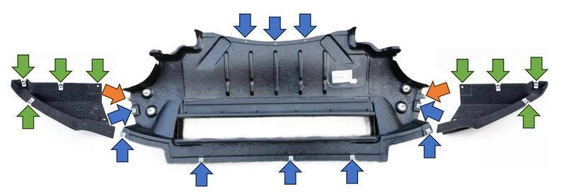
2. On the new undertray, add the supplied rubber trims to both sides of the inside edge, as shown.
