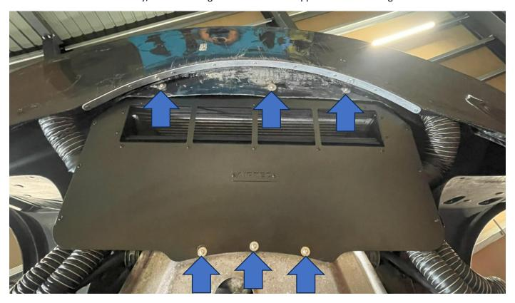
4. Slide the side sections into place and use the supplied M5x16mm bolts with washers to attach each side to the centre section but do not fully tighten yet. Then work around the edges fitting the remaining bolts and washers. The very outer edges of the side sections use the two larger remaining M6 bolts with larger 25mm washers. Once they are all in place, fully tighten all the fittings.
