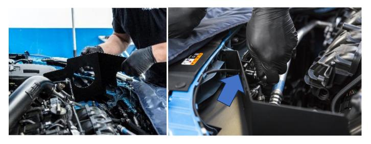
9. Once happy with the shield fitment, plug the MAF sensor back in position on the crossover pipe.
