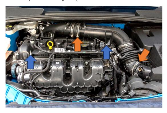
4. Loosen the jubilee clip securing the other side of the rear crossover pipe to the turbo. Before removing the pipe from the car, you will also need to release the breather hose attached to the back of the pipe (blue arrow).
