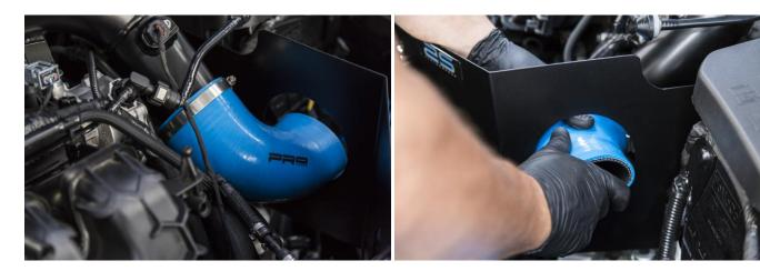
11. Install the supplied air filter onto the silicone hose with a jubilee clip, as shown.
