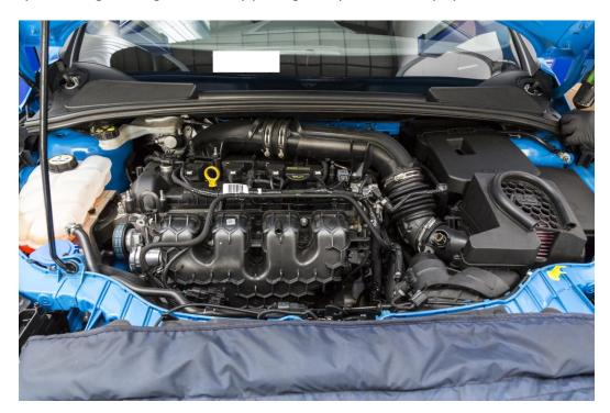
2. Disconnect the MAF sensor located on the original plastic hard pipe.
