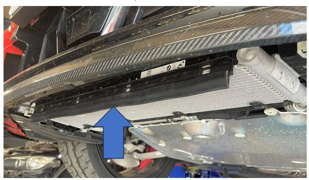
5. Finally, reinstall the AIRTEC Motorsport undertray and the rubber bumper trim removed in Step 1 in reverse of removal. All fittings are reused and locate in the same place.
