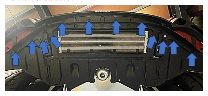
2. Release the undertray by removing the 14 10mm bolts securing it in place
