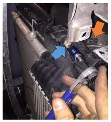
14. Now remove the standard plastic air guides either side of the radiator. These are not reused.
