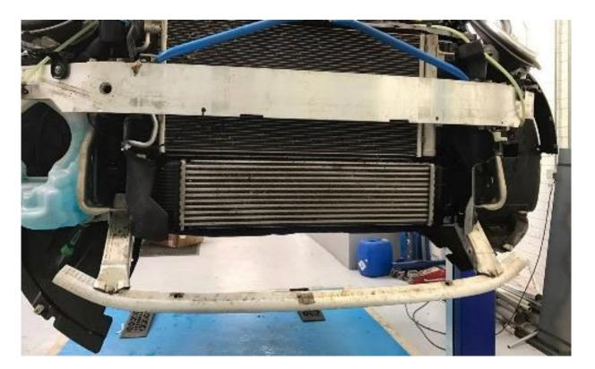
10. Unclip the bottom of the original intercooler using a flat-bladed screwdriver, as shown.
