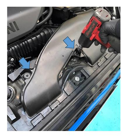
8. With the bumper off, remove the three bolts from each side of the lower crossmember/bumper support along with two bolts holding the plastic air guides to the crossmember.
