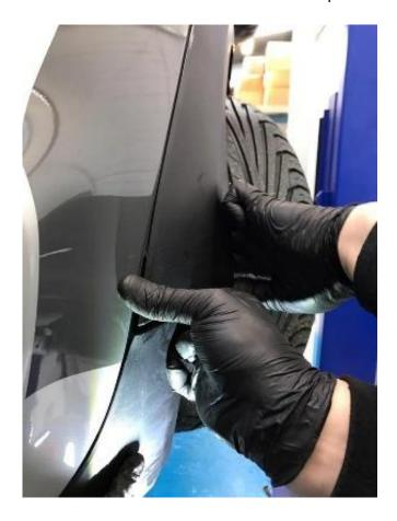
4. With the arches loosened, remove the T30 Torx bolt between the arch extension and bumper.
