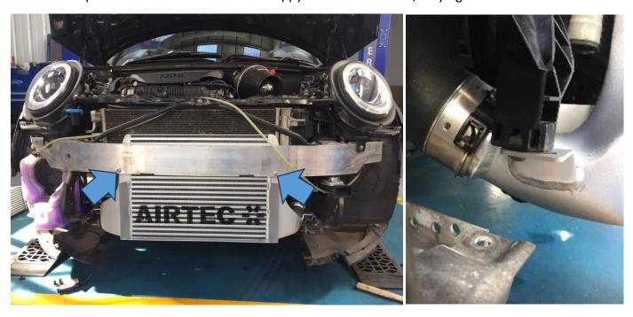
16. Finally, refit the lower intercooler mount removed in Step 11 using the supplied nuts, bolts and washers. Then refit the crossmember, bumper and undertray in reverse of removal.
