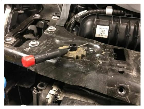
12. To remove the lower mount, you will need to drill out the four rivets securing it in place underneath. Please note: when installing the new intercooler, replace these rivets with the M6 nuts, bolts and washers supplied.
