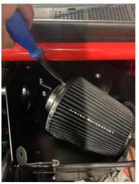
16. Now remove the MAF sensor from the old intake pipe and install into the new pipe using the two T20 bolts with washers supplied. Then reconnect the MAF sensor plug, shown.
