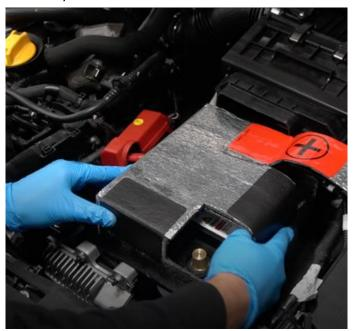
4. Remove the three bolts securing the battery tray in place using a 13mm socket. Then remove the two bolts securing the ECU bracket using a 10mm along with the additional two bolts from the side of the battery tray.
