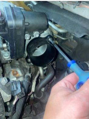
10. Install the silicone hose onto the new turbo intake pipe together with the supplied jubilee clip, but do not fully tighten to allow adjustment. Then install the front hose removed in Step 8 and replace the original clip with a jubilee clip (please note, the car shown has red hoses fitted).
