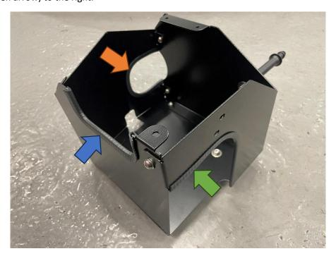
14. You can now install the AIRTEC Motorsport air box in place by fitting the two supplied locating pegs into the car's rubber mounting points. Once the position is correct and level, fully tighten the bolts.
