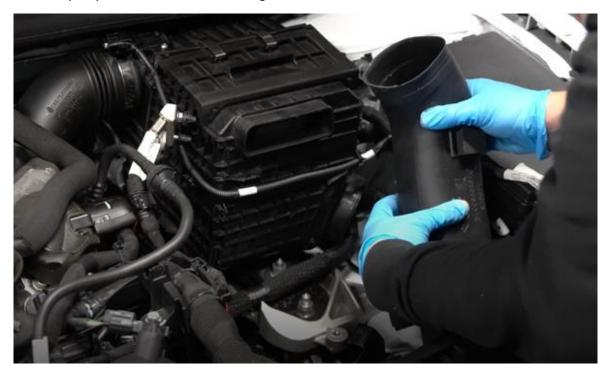
6. The MAF sensor can now be unplugged (blue arrow) and you can use either a 7mm socket or hose driver to release the clamp which is securing the original intake hose to the air box.
