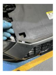
3. Undo the six T27 Torx bolts that are underneath, four in the middle and one either side.
