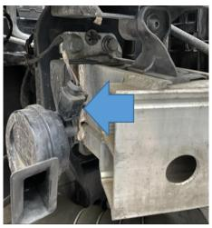
12. Remove the two T27 Torx bolts holding the plastic bracket to the front of the car.
