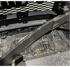
18. Now remove 16 T20 Torx bolts holding in the rear plastic support (four along the top, four each side and then four along the bottom). Once undone pull from both sides and it will release.
