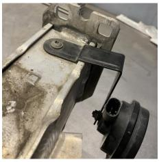
15. Before fitting the new intercooler, fit the two brackets facing forwards with the supplied bolts and washers, as pictured. Leave the bolts loose at this stage to allow adjustment when fitting.
