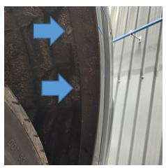
6. Now pull the arch extension away from the body by twisting the lower edge outwards whilst reaching behind and pushing in the centre of the plastic clip (highlighted with blue arrow), which will release the lowest point of the extension. Repeat this working up the arch until you have access to the Torx bolt holding the bumper to the wing. You can see the clips that you need to push in blue and the other clip is the one you have to twist the arch extension out to release.
