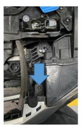
4. Underneath the car now, remove the six T20 Torx bolts along the underside of the front bumper.
