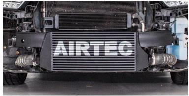
You can now refit the bumper to the vehicle, however we recommend for increased airflow and maximum performance to follow the below steps to remove the centre section of the grille that blocks some of the airflow.
