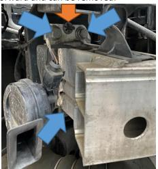
14. Remove the T20 Torx bolts securing the horns to the original crash bar and fit to the rear mounting bosses on the AIRTEC Motorsport crash bar.
