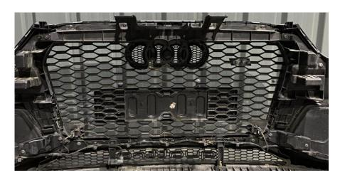
21. Finally, the bumper can then be reinstalled in the reverse of Steps 2 to 7. Please note; when reattaching the arch extension removed in Step 6 you may need to lift the back corner of the bumper over the inner lip to get the clips to fully seat home.
