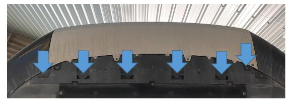
5. Inside each arch liner, remove the five T20 Torx bolts highlighted.
