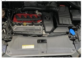
2. Remove the front upper panel by lifting at the edge and then pull the panel out.
