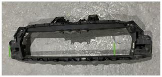
20. The surround can now be reinstalled using 14 of the original fixing to hold it in place.
