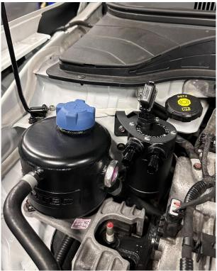
4. Finally, remove the original breather hose from the vehicle using a pair of hose clamp pliers. The new supplied hoses can then be installed as shown and secured with the supplied jubilee clips. Use the supplied hose separator to position the hoses. The engine cover can then be reinstalled.
