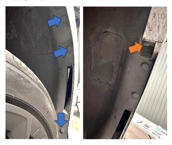
4. Using a second person to help, the bumper can now be removed. Start by pulling it away from the corners and then unhook it over the front panel. You will need to unplug a wiring connector on the left=hand side.
