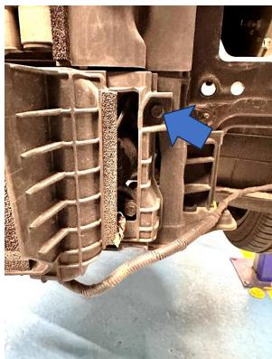
7. Next, the hot side boost hose can be removed using a pair of pliers to remove the protective caps from both the jubilee clips. Then loosen the clips and the hose can be removed from the car.
