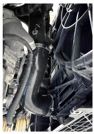
13. Before reinstalling the crash bar, the metal tab that held the air temperature sensor in place (removed in Step 5) will need to be removed. Use an angle grinder with a cutting disc (or similar) and appropriate PPE to trim the tab flush with the crash bar and then clean and paint the area with black paint to protect it.
