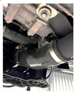
11. Install the new intercooler by angling it into the hot side boost hose first. Once located, secure the intercooler using the supplied four M6 bolts with washers.
