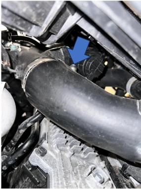
9. Remove the four remaining 10mm bolts securing the intercooler to the front panel and you can then carefully lift it from the car.
