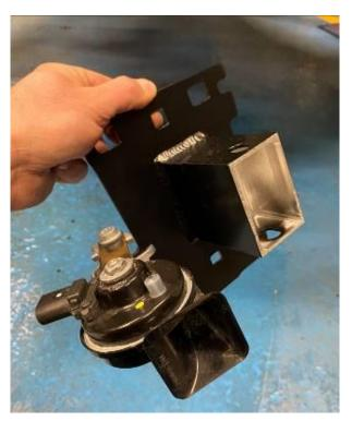
16. Fit the new crash bar feet reusing the original bolts removed in Step 13 but do not fully tighten at this stage.
