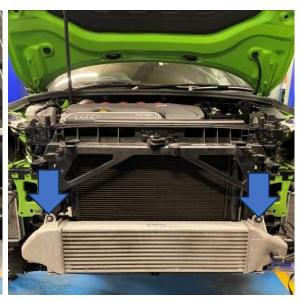
14. Undo the lower brackets by removing the T27 bolt each side.
