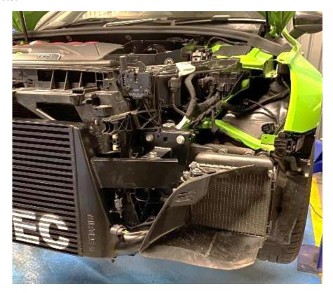
20. Finally, reinstall the air temperature sensor, auxiliary radiator guides, reconnect the horns and reinstall the headlights. The upper and lower air guides are not refitted. The bumper can then be reinstalled in the reverse of removal.
