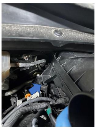
7. Remove the engine cover mounting posts from the car by undoing the 10mm bolts. Then install the two M6x16mm Socket Head bolts with washers where the post were to resecure the wiring harness.
