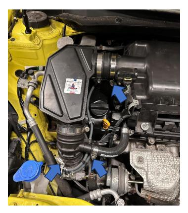
5. Unplug the MAF sensor and unclip the wiring harness to thew left-hand side of it.
