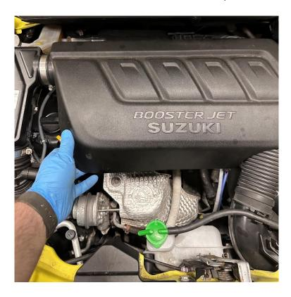
2. Remove the hose going to the coolant bottle and tuck it out the way, there may be a little coolant that spills as you disconnect it.
