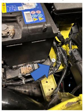
9. The induction shield can now be positioned in place. You will need to angle the front down as you move it into position and then install an M6x16mm Socket Head bolt with washer through the hole at the back and into the threaded spacer. The coolant hose removed in Step 2 can now be reinstalled through the hole in the induction shield.
