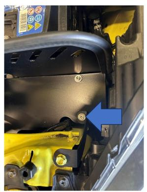
11. Now install the left-hand side bracket using the four M6x16mm Socket Head bolts with large washers as pictured. Once happy with the induction shield position, proceed to tighten all the bolts.
