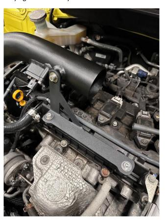
15. Fit the supplied silicone hose onto the MAF pipe as shown and then place the air filter in the induction shield. Position the remaining pipework through the induction shield and locate into the filter. The other end can then be fitted to the silicone hose with a jubilee clip but do not fully tighten yet.
