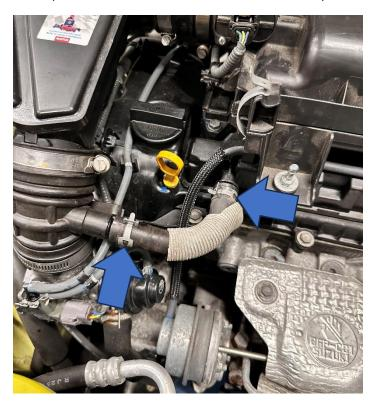
2. Finally, install the new silicone hose onto the car and use the supplied jubilee clips to secure in place.
