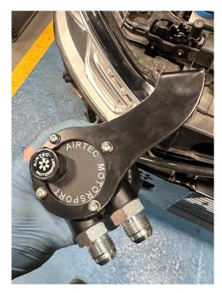
7. Install the bracket onto the car by using the supplied M8 bolt with washer into the spare thread, as shown.
