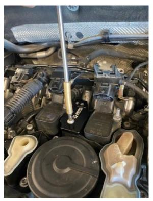
5. Undo the T27 Torx bolt (blue arrow) holding the turbo elbow to the car and release the wiring loom clip. You can then rotate the pipe (orange arrow) anti-clockwise to release it, which makes it easier to install the supplied push-fit to AN10 adaptor. Use the supplied clip to secure.
