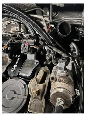
9. Install the two line separators supplied as shown, so that the lines are kept together and clear of anything that they may potentially foul on.
