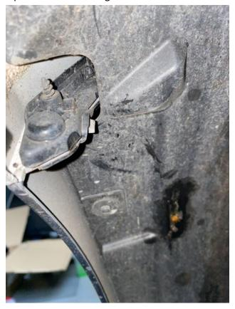
5. Carefully pull back the weather strip along the top of the bumper and remove the six T30 bolts underneath.
