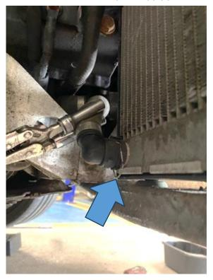
10. Release both coolant hoses from the radiator and make sure to have something in place to catch the excess fluid. You can then undo the single T27 bolt securing the radiator at the top and remove the radiator by lifting it from the bottom rubber mountings it rests on.
