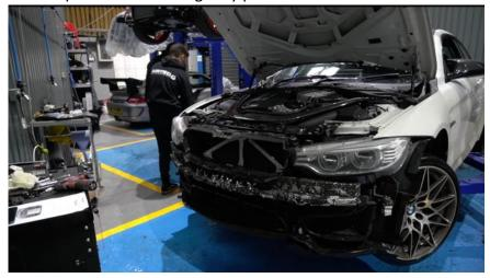
8. Now remove the air duct in front of the radiator you are replacing. Use a trim removal tool to release the two trim clips from the top of the guide and one from the bottom. Once they have been removed you can slide the air guide off the radiator.
