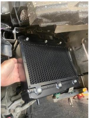
12. Once the new radiator is in place, you can reinstall the two coolant hoses in reverse of removal. Make sure you remove the original O-rings inside the hose fittings and replace them with the AIRTEC Motorsport supplied O-rings before reconnecting.
