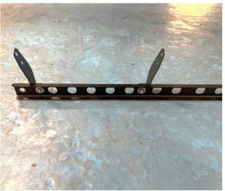
7. Bolt the new brace assembly in place reusing the original bolts removed in Step 4.
