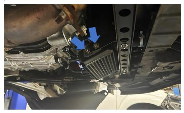
9. Attach the two supplied silicone hoses with four jubilee clips to the gearbox cooler, exactly as shown **but do not tighten.** The shorter hose (blue arrow) fits to the nearest side of the gearbox cooler in the orientation shown and the longer hose (orange arrow) fits to the furthest side in the orientation shown.
