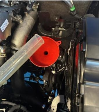
14. Please read carefully: If safe to do so, we now recommend starting the car whilst the wheels are still off the ground and running it up to temperature whilst in gear to ensure the gearbox oil circulates around the new oil cooler and lines.
