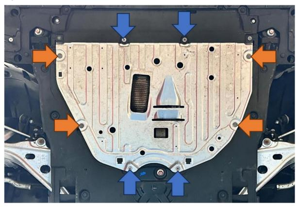
2. Remove the plastic trim panel further forward by releasing the eight fixings.
