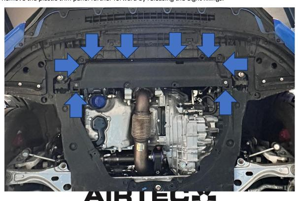
3. Remove the fittings holding the lower right-hand side part of the undertray in place **without** fully removing the whole undertray in order to gain some extra clearance when fitting the gearbox cooler. There are clips inside the inner wheel arch liner that also need removing before it can be folded down, as shown.
