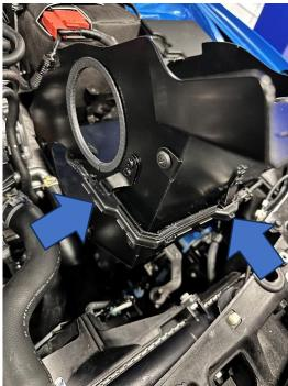
11. Remove the MAF sensor from the original air box using a Phillips screwdriver to release the two screws holding it in place. Then install the sensor into your new induction pipe using the supplied M4 bolts.
