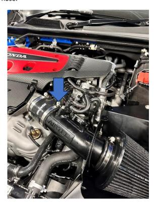
16. Install the top of the air box using the five remaining plastic push fittings, followed by fitting the supplied rubber trim along the front lip to seal it, as shown.
