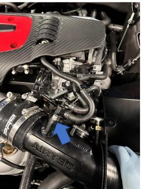
13. Now fit the air filter onto the end of the pipe. You will need to angle the filter as shown to get it to slide onto the pipe. Once happy with the fitment, fully tighten the jubilee clip.
