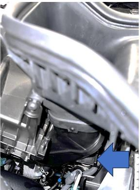
8. Install the new Pro Hoses silicone connector onto the inlet pipe and reattach the vacuum line removed in Step 2 using the supplied jubilee clips to secure in place. Once happy with the orientation, fully tighten the clips.
