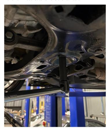
${\bf 4.} \quad {\bf Undo\ the\ three\ 16mm\ front\ bolts\ to\ release\ the\ front\ bracket}.$
