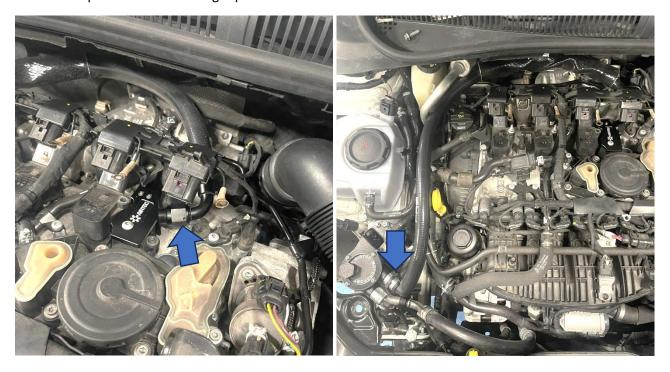
10. Install **Hose B** by fitting the 45-degree push-fitting into the turbo elbow removed in Step 3. Route the hose in the same way and then connect the final push-fitting into the catch can. Make sure the heat protection is in the right place over the turbo.
