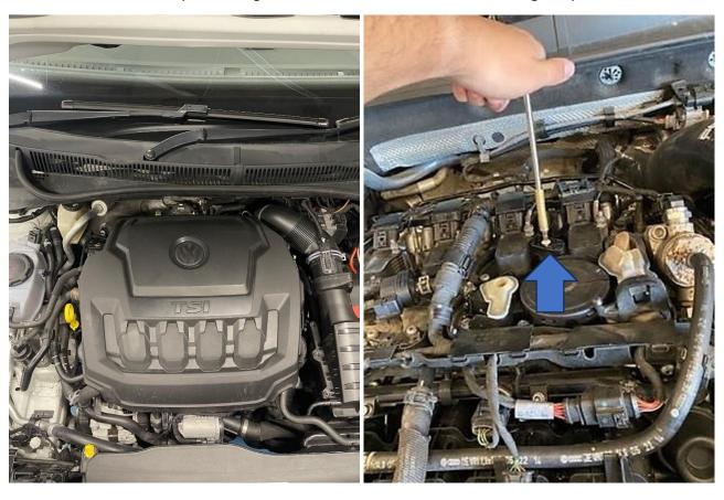
2. Remove the four 10mm nuts securing the wiring harness for the coil packs in place. Once undone, you can unplug the coil packs and the harness will lift enough to allow access to the breather outlet.
