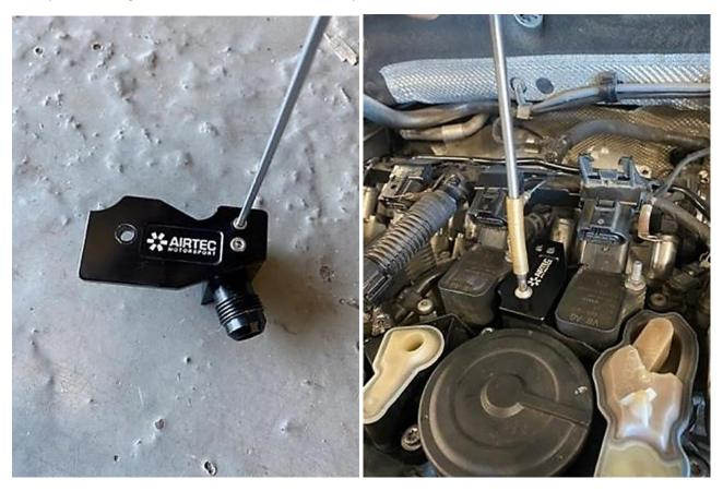
5. Install your AIRTEC Motorsport catch can onto the bracket as shown using the four supplied M5 bolts with washers.
