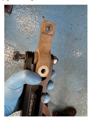
4. Install the torque mount to the car reusing the original bolt at the rear.
