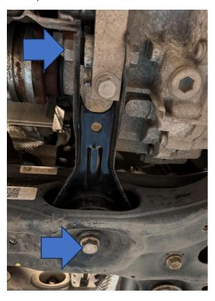
2. Now undo the two 14mm bolts holding the bracket to the engine and then rotate it down enough so the centre bolt can be removed from the torque mount. You can then remove the torque mount from the car. Please note: You may need to rock the engine towards the front of the car to release the mount.
