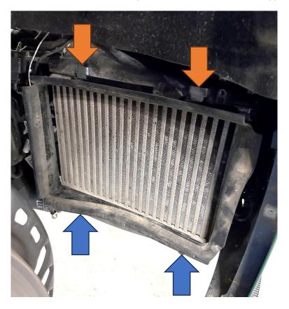
5. Undo the jubilee clip holding the lower boost pipe in place and remove the hose from the intercooler.
