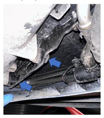
7. Lift the intercooler up by pushing gently from underneath to release the three mounting pins from the rubber mounts attached to the car. As you pull the intercooler back to remove it from the car you will be able to access the front air guide, which you need to remove it from the intercooler in the same way as the rear guide. You can then leave the guide in place on the car.
