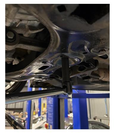
4. Undo the three 16mm bolts in the gearbox to release the front bracket.
