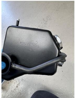
6. Finally, refit the hoses and install the new tank onto the vehicle reusing the original 10mm bolts. Then reinstall the brackets removed in Steps 1 to 2. You can then top up the tank with coolant as necessary.
