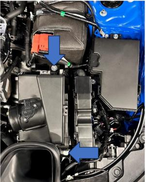
4. The wiring harness to the battery will need to be unclipped using a trim removal tool or flat-blade screwdriver.
