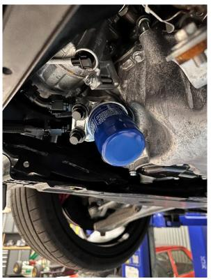
17. As the lower oil line passes by the protruding bolt highlighted, add the supplied conduit plastic shielding.
