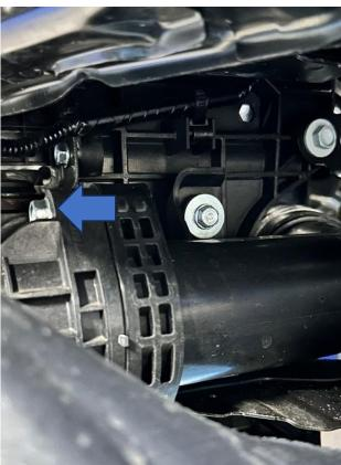
8. Now remove the two 12mm bolts holding the intercooler flange to the boost pipe flange each side and remove the intercooler from the car.
