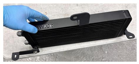
11. Remove the bolt in the centre of the front panel, as highlighted. The oil cooler can then be passed up from below the crash bar and secured in place by reusing the same bolt to attach the oil cooler's top bracket to the car.
