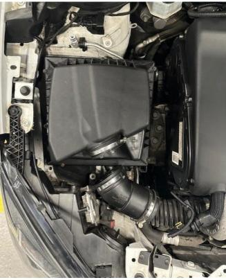
2. Now remove the air box from the car. It is held in with rubber push fittings at the front and back, which will release with a small amount of force.
