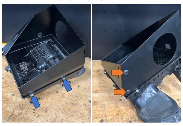
6. Attach the small rubber trim provided around the hole in the induction shield (blue arrow). Place the larger rubber trim and place it around the induction shield top (orange arrow).
