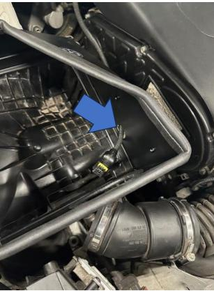
8. Push the original induction pipe into the air box and refit the MAF sensor pipe using one of the original jubilee clips. You can then reconnect the MAF sensor plug.
