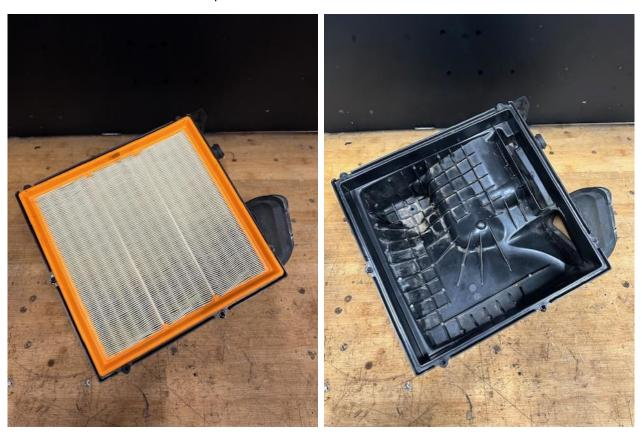
4. Place the main part of the induction shield onto the air box base, as shown. Use four of the supplied screws with washers to secure it in place.
