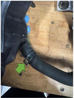
8. On the other end of the larger hose you just removed from the reservoir, use a Dremel tool or similar to cut through the metal clip securing the 90-degree fitting and remove it from the hose. Place the fitting aside as it will be reused when installing the new AIRTEC Motorsport chargecooler.
