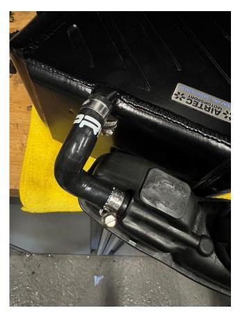
11. Fit the larger supplied replacement silicone hose to the underside with the 25mm jubilee clip provided
