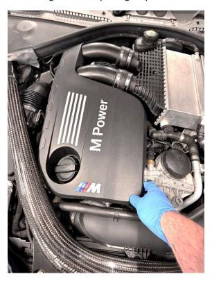
2. Undo the three jubilee clips securing the silicone couplers on either side of the original chargecooler using and remove them.
