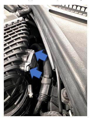
4. We recommend clamping the hoses using a suitable hose clamps in the two locations shown, otherwise you will need to drain the coolant for the chargecooler circuit. We also suggest placing a cloth underneath the connectors to try and collect any spilt coolant in the later steps.
