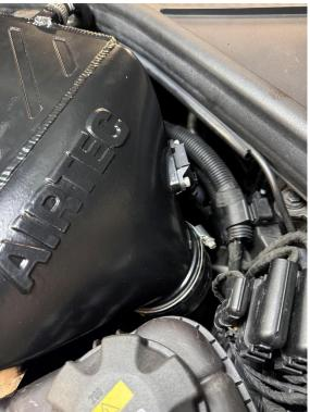
13. Install the 90-degree fitting removed in Step 8 on to the other end of the hose larger silicone hose using with the supplied 25mm jubilee clip and then reattach all three water connectors.
