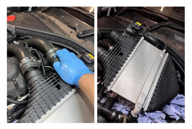
6. With the chargecooler now free to move, use a small pick tool or flat-blade screwdriver to lift the spriong clips for the three water connectors and remove then, whilst tilting the chargecooler back, remove it from the car. Drain the coolant from the chargecooler into a suitable container.
