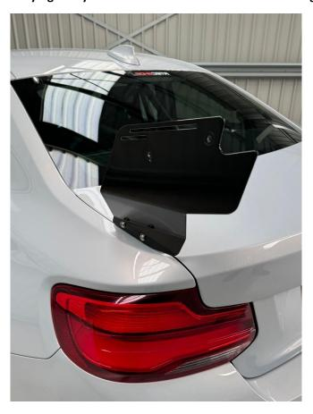
5. Repeat the previous steps on the opposite side. Once complete, mount the centre blade in place using the supplied M6x20mm Button Head bolt with small M6 washers.
