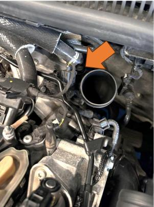
4. Rotate the elbow clockwise approximately one third of a turn and it will release from the turbo.
