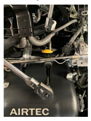
19. You can now start to reinstall the coolant lines, the wiring harness and MAP sensor that attach to the throttle body elbow along with tightening the jubilee clip. The alternator wiring can be reattached, along with the throttle body and plug removed in Step 8.
