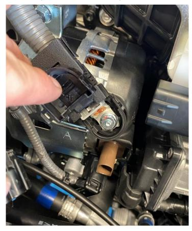
4. Undo the 10mm nut (blue arrow) and then release the clip (orange arrow) holding the wiring harness in place and fold it backwards over the engine so it is out of the way.
