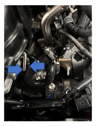
13. The manifold can now be lifted out of the engine bay. Once it is on a bench, the throttle body and elbow can be removed by undoing the four 10mm bolts securing it to the manifold.
