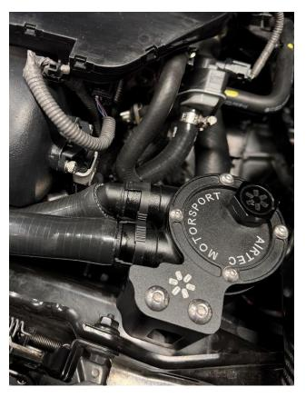
27. Ensure all plugs are connected and clips/clamps fully tightened.
