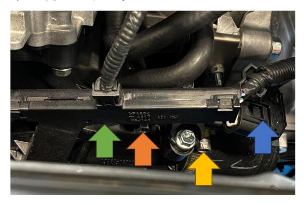
11. Undo the two 12mm nuts and two 12mm bolts to loosen the inlet manifold. The throttle body has coolant lines going to it and so the inlet manifold cannot yet be fully removed from the car at this stage.
