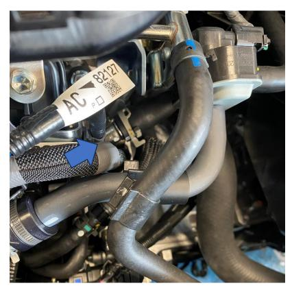
6. Undo the three 10mm bolts (blue arrows) holding the coolant hard pipe above the inlet manifold and move the hard pipe back so that it is out the way. Then, on the lower right-hand side, locate the wire and plug (orange arrows) and disconnect it by pushing the blue button and pulling it backwards.
