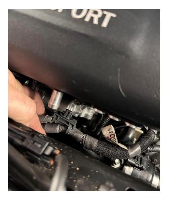
21. Reinstall the coolant hard pipe onto the tabs on the inlet manifold, re-using the original bolts. It will no longer bolt onto the right-hand side.
