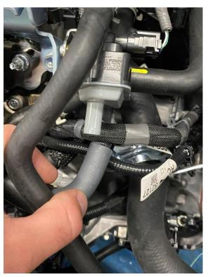
9. Now **loosen but do not fully remove** the 12mm bolt (blue arrow) and **remove** the second 12mm bolt (orange arrow) securing the throttle body elbow in place. The bracket should then move down out of the way. You can then unplug the throttle body wiring.
