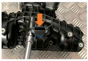
15. Now refit the gaskets to the new manifold and secure the MAP sensor (blue arrow) to the side of the manifold using the supplied M6x12mm bolts with washers. If you are not using of the NPT ports underneath the manifold, then please ensure that the supplied NPT plugs are fitted tightly (orange arrows).
