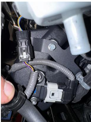
25. Disconnect the one-way valve from the breather hose removed in Step 8 and refit it to the supplied silicone hoses. It can then be fitted back onto the car with the supplied jubilee clips, as shown. **Please note:** The direction of the one-way valve is important: make sur the arrow points on the valve points **towards** the inlet manifold.
