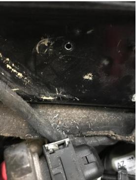
6. Secure the breather tank to the bulkhead with the supplied self-tapping bolt.
