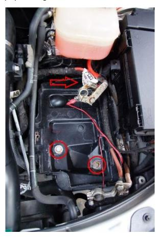
4. With battery tray removed, remove the original plastic breather fitting (blue arrow). Then remove the gearbox fill plug (orange arrow) and replace with the supplied barbed fitting.
