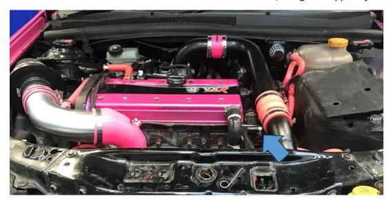
4. Fit the shorter silicone hose to the top outlet of the turbo cooler and connect it to the turbo side removed in Step 3, using the supplied jubilee clips.
