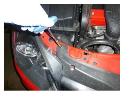
2. Bolt the mounting bracket to the cooler using the bolts and washers as shown (blue arrows). Then offer it up to the edge of the slam panel by the bonnet catch and mark the two holes (orange arrows). Drill using a 6mm bit and then secure the bracket in place using the supplied bolts, nuts and washers both sides.
