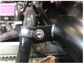
6. Finally, run the car up to operating temperature and check for any leaks. Once happy, top up the coolant as necessary and refit the top grille in reverse of removal.
