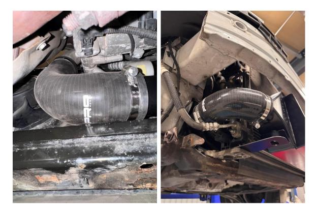
21. Ensure all fixings and clips are tight and then all parts can be reinstalled in reverse of removal - **except for the two side air guides removed in Step 7.** The left-hand side guide cannot be reinstalled and the right-hand side guide needs to be cut, as shown, before it can be reinstalled.
