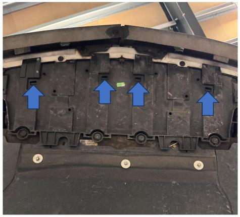
4. Once the undertray is removed, in each corner locate the E12 Torx bolt and remove it.
