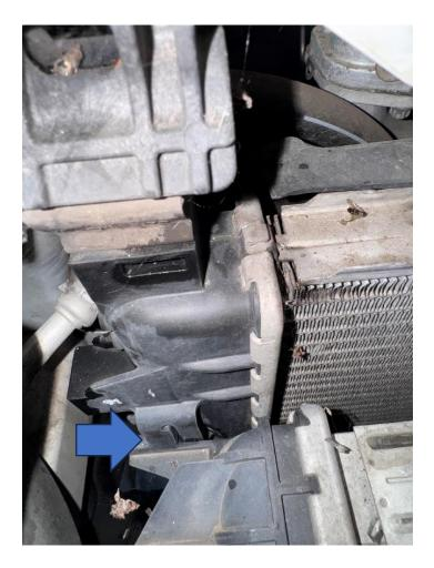
12. Reinstall the air-con radiator onto the mountings on the radiator that used to hold the intercooler.
