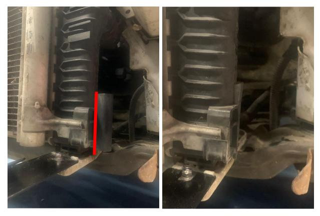
17. Install the centre bracket onto the intercooler using the supplied M6 fixings and then hang the intercooler on the crash bar. Use the supplied M4 bolts with Nyloc nuts with washers to go through the existing holes in the crash bar and tighten to secure, as shown.
