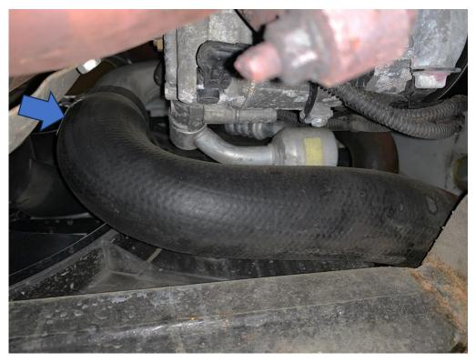
15. Now unbolt the air flow sensor (blue arrow) and then remove the entire pipe (orange arrow) by disconnecting it at either end. There is also a bolt holding the pipe in place by the front panel (green arrow).
