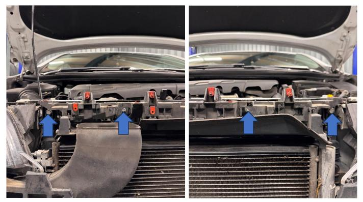
9. Undo the 10mm bolt securing the lower air feed and then pull it towards the front of the car to allow the upper radiator air guides to be removed.
