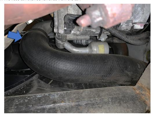
15. Now unbolt the air flow sensor (blue arrow) and then remove the entire pipe (orange arrow) by disconnecting it at either end. There is also a bolt holding it in place by the front panel.
