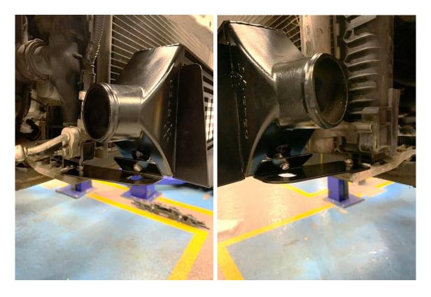
19. Route the cold side pipework with the supplied jubilee clips. Then refit the air flow sensor removed in Step 15 and once happy with the positioning of the hoses and pipework, tighten all jubilee clips.
