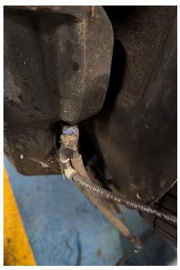
6. Remove the upper air box feed by undoing the two T25 Torx bolts.
