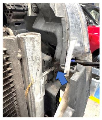
11. Under the car, remove each of the standard boost pipes from the intercooler by releasing the clips using a flat-blade screwdriver. Then unhook the intercooler from the radiator and lift it upwards and out. Take care not to damage the fins on both the air-con radiator and water radiator.
