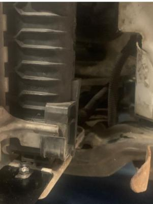
17. Install the centre bracket onto the intercooler using the supplied M6 fixings and then hang the intercooler on the crash bar. Use the supplied M4 bolts with Nyloc nuts with washers to go through the existing holes in the crash bar and tighten to secure, as shown.
